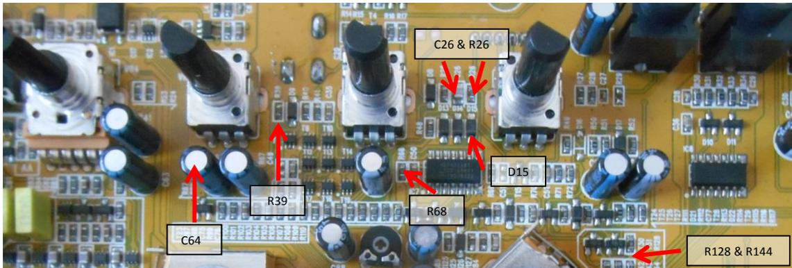
**Variable Accent decay** (adapted from Xobox wiki): lift top of D15 (= anode of OG D28), and wire a 1M log potentiometer between the lifted top and the freed solder pad on the PCB. Alternatively cut the trace between PIN3 of the decay pot and the top of D15. For simple fine-tuning of accent decay rather than variable decay, use a resistor or a trimmer. NB that the accent decay can never exceed the decay as set by the main envelope.
