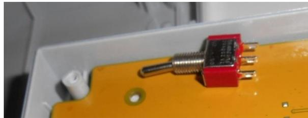
Top: You have enough space for an insulated solder lug potentiometer or horizontal print potentiometer in places where there are no capacitors underneath the chassis (see backside). There is plenty of space in the area of the Behringer logo underneath the led.
