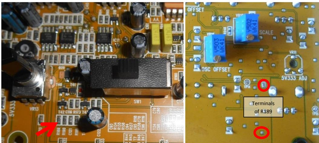
**Second wave input (easy version):** Firstly, note that the VCO signal is not buffered, i.e. always have some resistance in between and never fully ground it. If you don't want to
