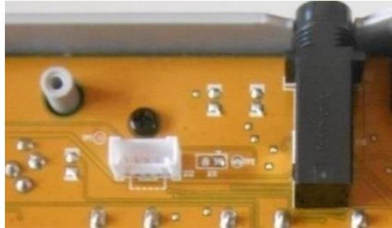
**Gate Input** (adapted from xobox wiki): Tip lug of input jack socket goes to 22k resistor. The other end of 22k resistor goes to a diode, the cathode of which goes to base of T30. The junction between T30 and R142 goes to a solder point on the **back of the PCB**. This only works when physical ground is connected (i.e. output/usb cable plugged or ring lug of your CV input socket connected to TP1 or Pin5 of X12).
