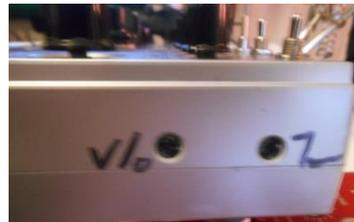
Sides: Components may be best placed underneath the PCB. You could implement trimmers (glued to the underside of the PCB) for resonance, V/OCT calibration and square wave pulse-width that can be accessed with a small screwdriver from little holes on the side of the chassis. This way you don't need to open the box if you want to make adjustments.
