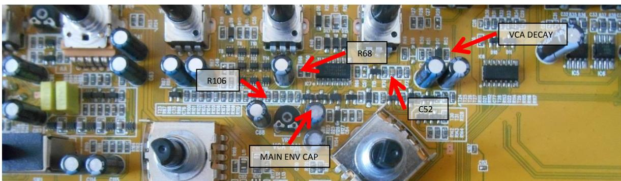
**Different speeds for main envelope** (xoxbox wiki): exchange C89 with capacitors of different values to taste. For folks who think the TD3 decay could be snappier, put in smaller cap values. Using a switch, you can toggle between speeds. Longer also makes accent swing in – I added 1uf to the existing 1uf with an ON-OFF switch.
