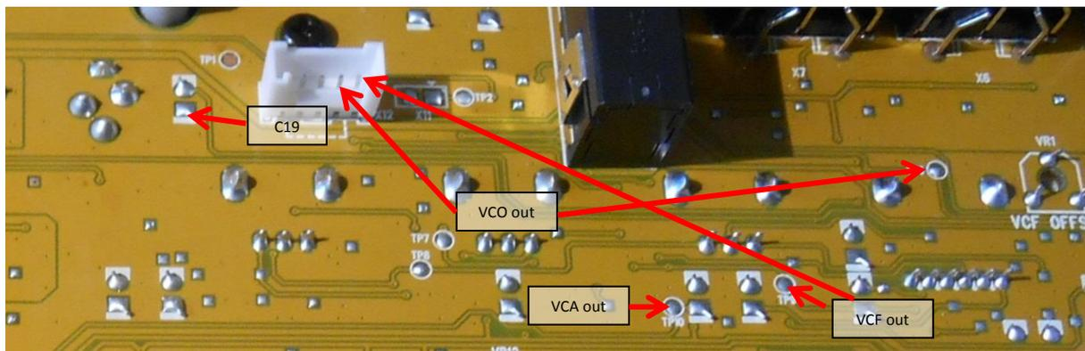
**Extended Filter mode:** wire TP6 to a switch, a 150k resistor and switch in series, and then to the bottom of R123 for phasey, bandpassy effects. This feeds the raw wave to a point after the ladder filter stages.
