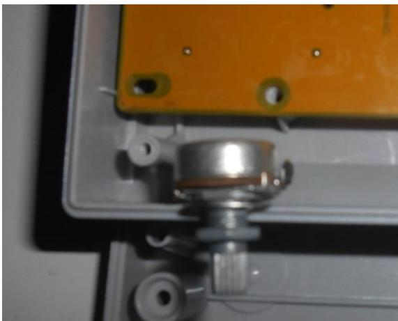
Front: Like on the RD8, there is quite some space between the PCB and the front of the chassis, which means larger components can be placed here most easily.
