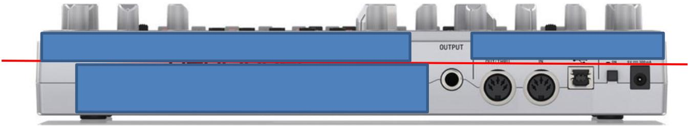
Red line indicates position of PCB. Areas marked blue fit components.
