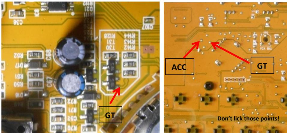
**1V/Oct CV input** (adapted from Doepfer): For proper V/Oct input wire to the bottom of R64 (or the point on the **back of the PCB** described in the VCO section) first a 27k resistor (Doepfer mistakenly wrote 7K) and then a 4.7k trimmer for fine-adjustment. If you have never calibrated VCO tuning, best check a (video) tutorial first – easy but takes patience.
