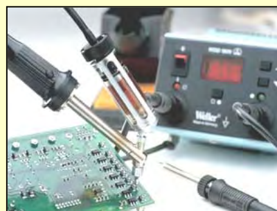
"Desoldering appliance": for easy desoldering of point solderings
