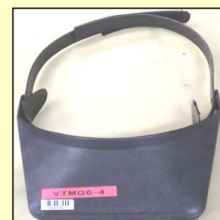
"Soldering magnifying glass": for a good view during soldering
