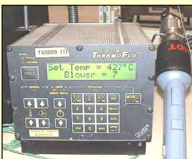
"Warm air desoldering appliance": for easy desoldering of flat-package IC's
