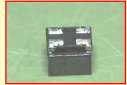
SMT component with contact surfaces beneath the component
