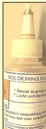
"Flux dosing bottle": for easy adding of flux (with brush)
