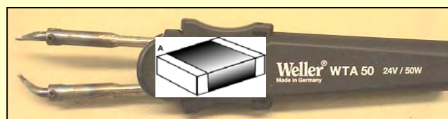
"Tweezer-copper bit": handy tool for the removal of SMD/SMT components.
