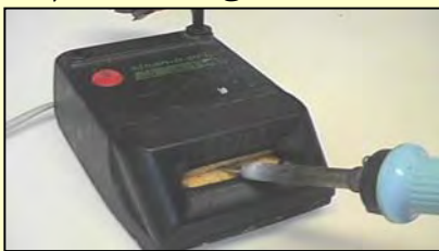
"Clean-o-point": for automatic cleaning of the soldering bit with 2 rotating sponges
