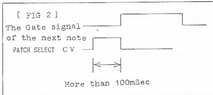
The Fig 2 shows how the GATE signal and the PATCH PRESET CV should be input. If the pulse is shorter than 100mSec, a kind of noise might be heard.
