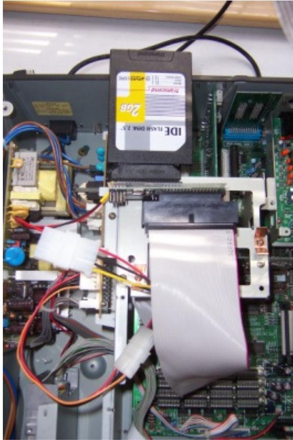
Below: Barely visible, but after powering up the unit, it recognizes the IDE as an Internal SCSI drive, and is showing 1.96GB free. Success!
